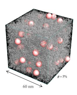
The state of dispersion of nanoparticles in polymers is key to the properties of polymer-matrix nanocomposites. In applications one strives to achieve a good dispersion by judicious molecular engineering design of the polymer matrix and filler nanoparticles and of the processing conditions used to form the nanocomposite.
